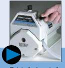
Rotate the lever to the right to close head. Adjust occlusion setting by turning knob on top of pump head.
