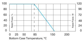
Best results can be obtained by using a thermal transfer compound with a heat conductivity of better than 1 W/mK. The flatness of the cooling plate must be better than 0.05 mm overall. Surface roughness should not exceed 6.4  $\mu m$ .
