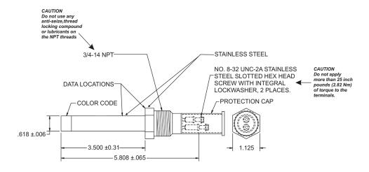
Figure 1. Fire/Overheat Detector
