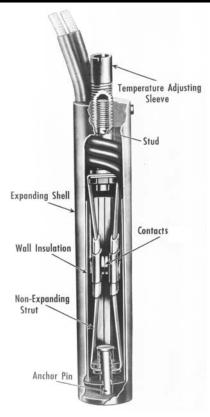
'to "lead" the struts by an interval that varies with the rate of temperature change. With rapid temperature rise, the shell exerts a larger net force on the struts and tends to pull them apart sooner than if the temperature were rising slowly. The result is several degrees or more of anticipation which helps produce closer control.
