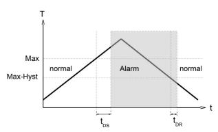
In the normal state the integrated LED is on, in the alarm state it is off, and this corresponds to its status when there is no supply
