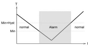
With a maximum-switch, exceeding the limit value causes a switchover to the alarm state. Return to the normal state occurs when the measured value once more falls below the limit value minus the set hysteresis.
