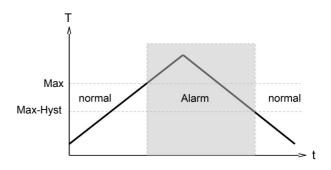
A switchover delay time (t<sub>DS</sub>) can be applied to the switchover to the alarm state. Equally, one switch-back delay time ( $t_{\text{DR}}$ ) of several can be applied to switching back to the normal state.
