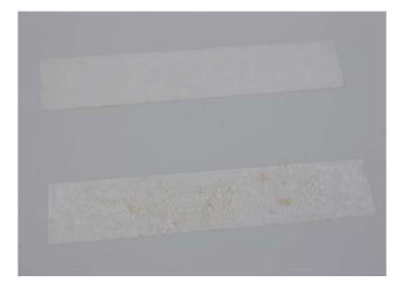
Clear tape is pressed on the measurement surface, torn away and stuck onto white paper - For reference a clean piece of tape is also stuck on the same white paper.
