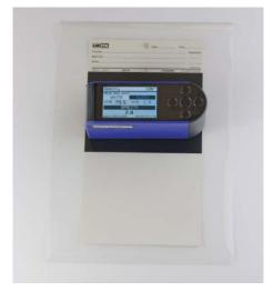
Measurements are made over a white substrate and then over a black substrate. Opacity is automatically calculated and displayed.
