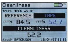
Fast measurement of all parameters Automatic calculation of cleanliness
