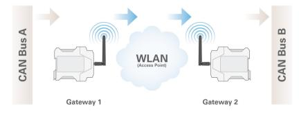
For unidirectional data transmission the message traffic from CAN bus A is to be forwarded to CAN bus B via a WLAN network. Necessary for this are two PCAN-Wireless Gateways and the creation of a route on each device.
