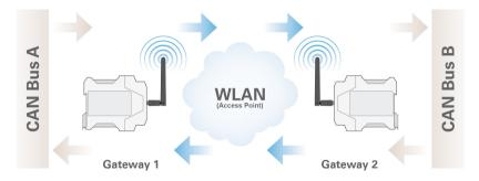
For bidirectional data transmission the message traffic occurring between CAN busses A and B is to be forwarded via the WLAN network. For this two PCAN-Wireless Gateways are needed, where for each one, a Send and Receive route must be created.
