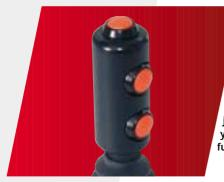
The cylindrical profile of the SW handle allows full grip use when controlling the JC400 range. 'Person present' switch functions can be incorporated by using a choice of three switch arrays which can offer a combination of finger and thumb activation. The external button switches can be used to verify the change in signals from the joystick, which may help to increase the integrity of your control system, or enable control of additional functions.
