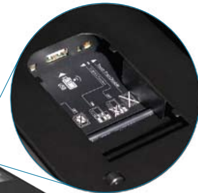
For even more convenience and versatility, the top of the keyboard/mouse tray features a hideaway USB port for USB HID-supported wireless keyboards and mice (RF or Bluetooth).
