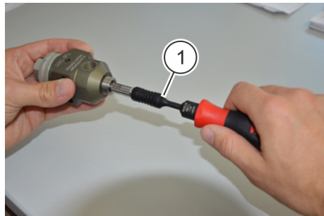
Fig. 18: Tightening the seal screw with torque screw driver
