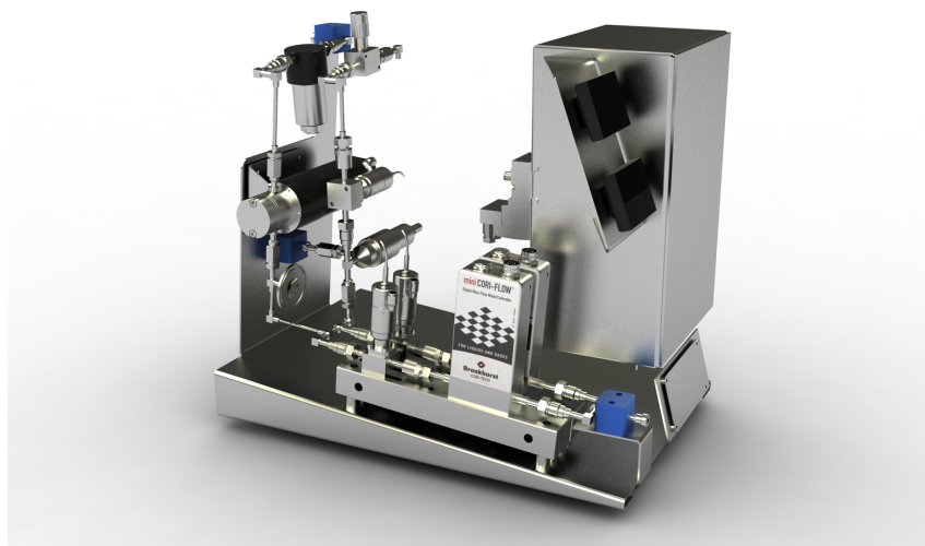
(a) 3D model of dosing skid
