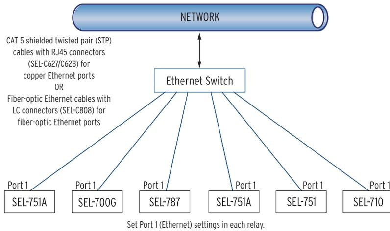
**Figure 10 Simple Ethernet Network Configuration**
