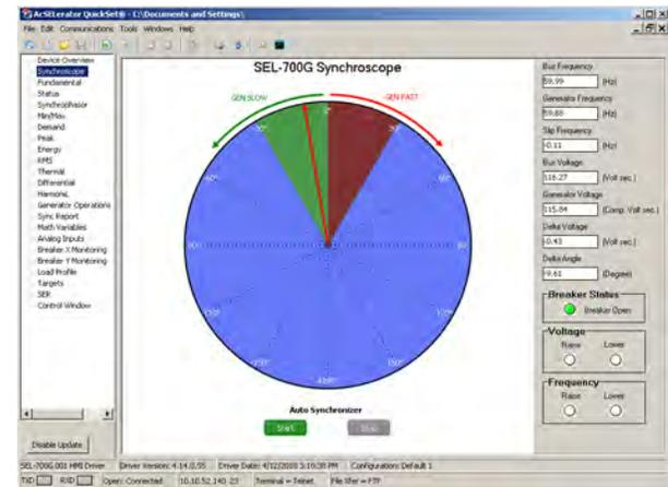
Figure 4 QuickSet Synchroscope
