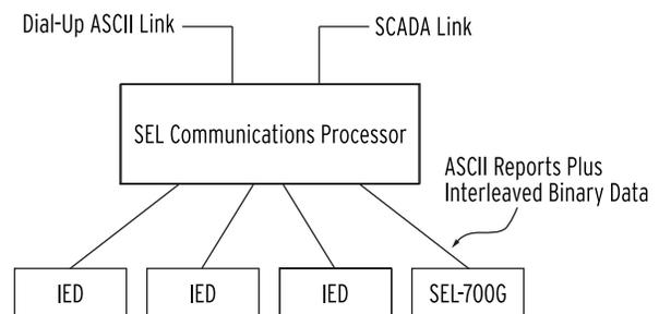
**Figure 9 Example Communications System**
