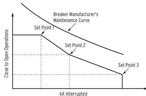
**Figure 8 Breaker Contact Wear Curve and Settings**
