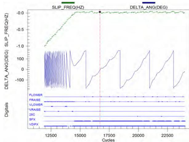
**Figure 7 Graphical Display of Generator Synchronizer Report**
