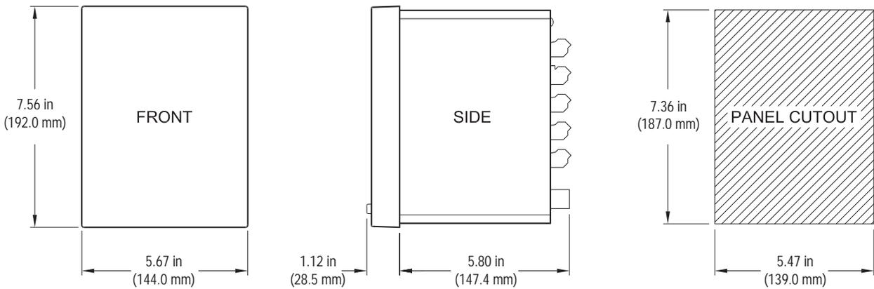
Figure 14 SEL-700G Dimensions for Rack- and Panel-Mount Models
