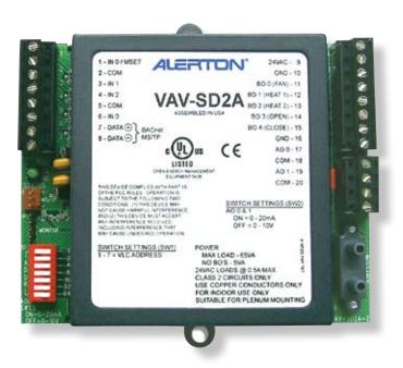
The Alerton® BACtalk® VAV-SD2A is a versatile, BACnet-compliant field controller that provides pressure-independent control of any single-duct variable air volume (VAV) box. It is particularly suited for controlling VAV series fan boxes equipped with a variable speed fan. As a native BACnet controller, the VAV-SD2A integrates seamlessly with your BACnet system, communicating at up to 76.8 Kbps on a BACnet MS/TP LAN. The VAV-SD2A-F includes a filter to reduce dust contamination.
