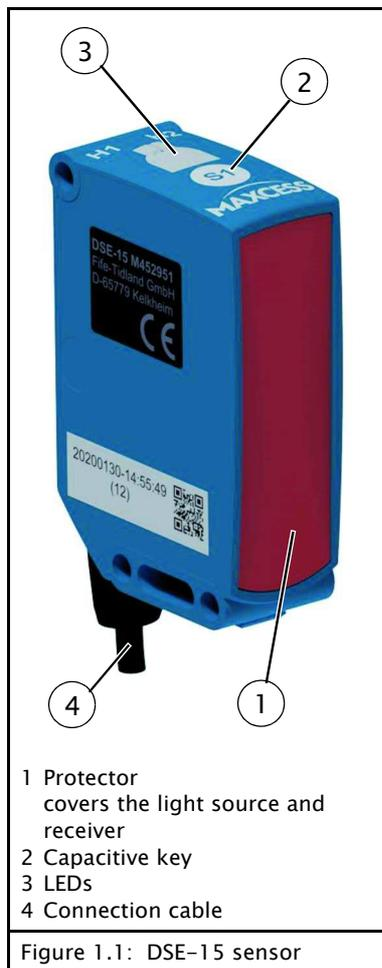
The DSE-15 sensor uses pulsing, visible red light for coaxially transmitted and received light beams. This makes the sensor insensitive to ambient light and reflections.
