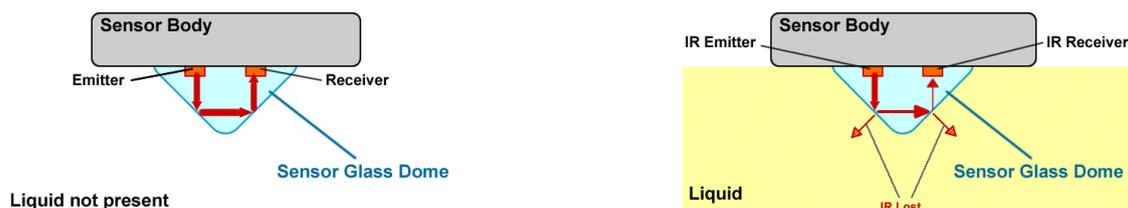
The sensors contains an infrared-ray emitter and an optical receiver. In air (liquid not present), all the light emitted is reflected - internally - by the dome and then redirected to the receiver. When the liquid reaches the sensor dome, a big amount of the light emitted is lost in the liquid and the sensor senses its presence.
