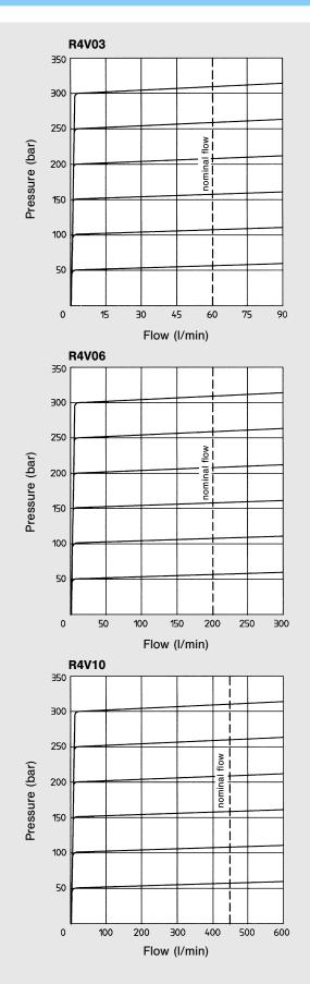
min. pressure setting  $\geq$  3 bar (depending on flow and viscosity). Fluid 40 cSt at 50 °C  $\pm$  0.5 °C.
