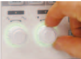
Dual knobs for vertical/horizontal manipulation of waveforms
