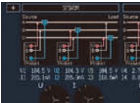
Wiring confirmation function, to avoid wiring mistakes
