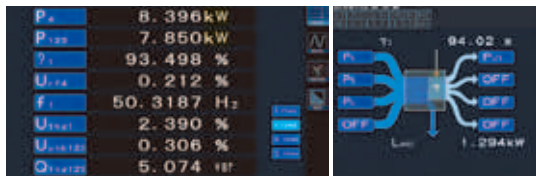
P4: DC power (panel output) P123: 3-phase power (power conditioner output) η1: Conversion efficiency Ur14: Ripple rate f1: Frequency Uthd1: Voltage total harmonic distortion Uunb123: Unbalance rate Qnd123: Fundamental wave reactive power
