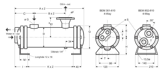
The oil and water connections can be chosen freely. The counterflow system remains due to our 4-way system. Standard connection on the oil side with BSP thread. DIN and SAE flange can be supplied upon request. Oil connections can be arranged laterally in reverse order upon request. The dimensions " C " and " B " cannot be changed.
